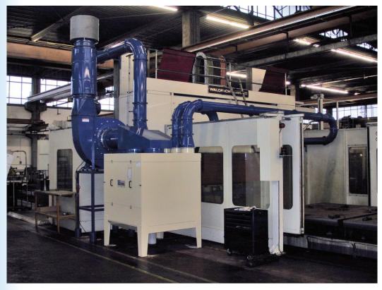
The Coral Oil Stop series mist collector/air filter is specifically designed for multiple machine tool applications to efficiently remove coolant mist, oil mist, smoke, and filter the air during machine tool operations.
